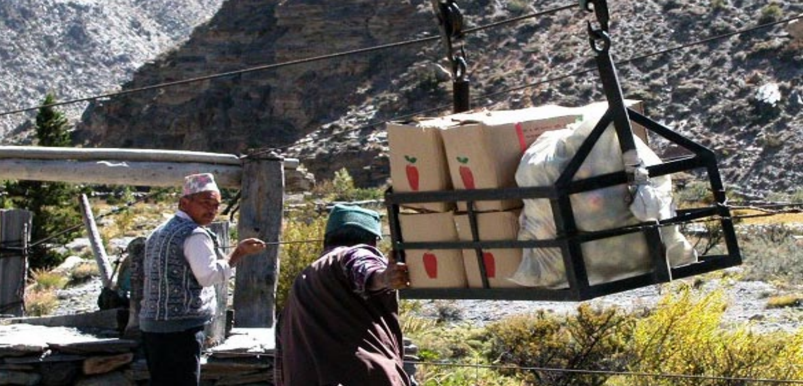
Transporting goods using a gravity ropeway.
